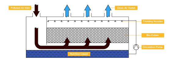
The biofilter system uses a combination of biological oxidation, adsorption, and absorption to remove odor and harmful gases from the air.
